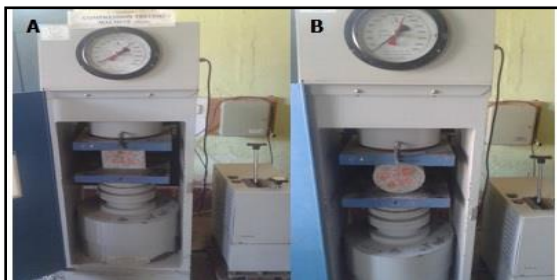
Figure 2. Testing of specimens, A. Compression test, B. Split tensile test.
