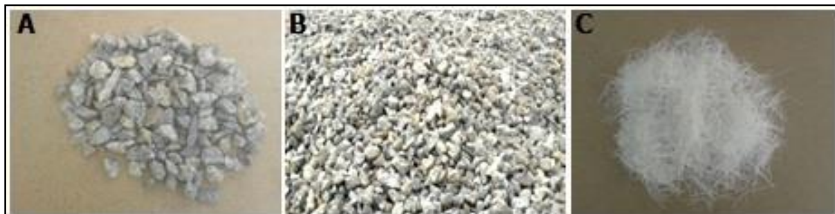
Figure 1. Materials, A. Natural coarse aggregate, B. Recycle aggregate, C. Polypropylene fibres.
